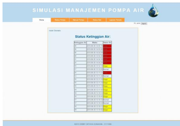
Fig. 5. Web interface for water level monitoring
