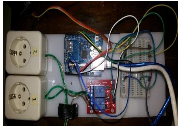
Fig. 4 Circuit design using arduino and relay board
