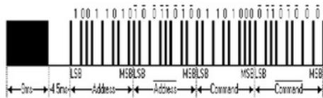
Gambar 2. Format Data Remote Control NEC<sup>[6]</sup>
