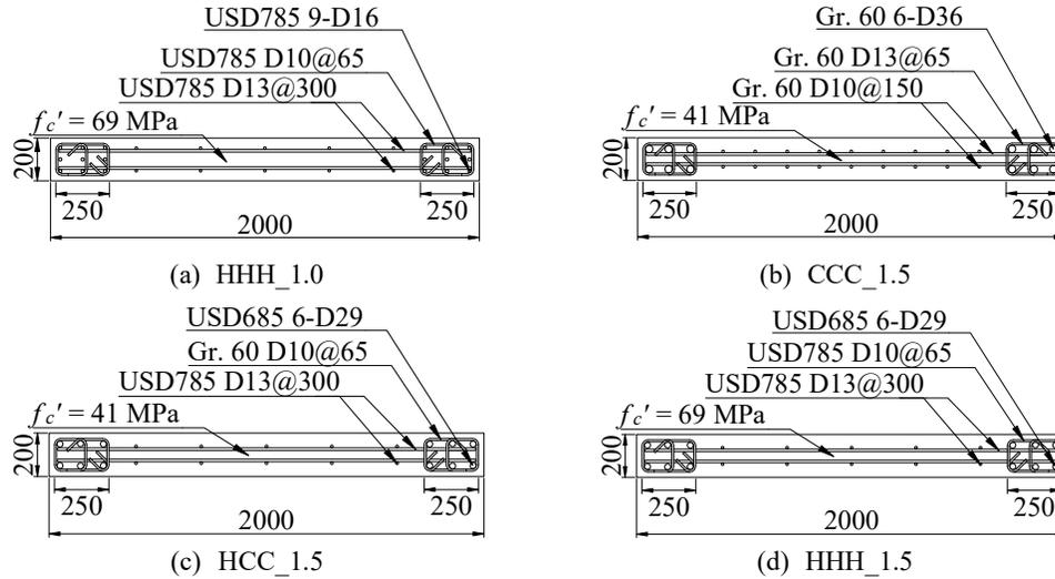
**Fig. 1 – Reinforcement Layout (unit : mm)**
