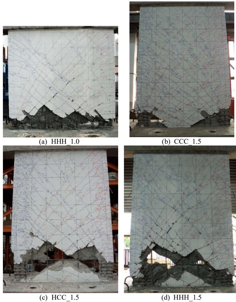
**Fig. 3 – Final States of Test Specimens**
