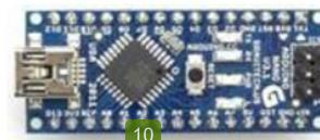
Gambar 1. Arduino Nano Board
